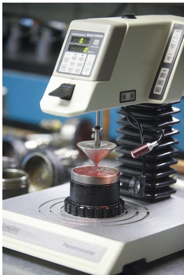
Figure 3. ASTM D217 (cone penetration test) evaluates the consistency of greases over the full range of NLGI numbers from 000 to 6.
